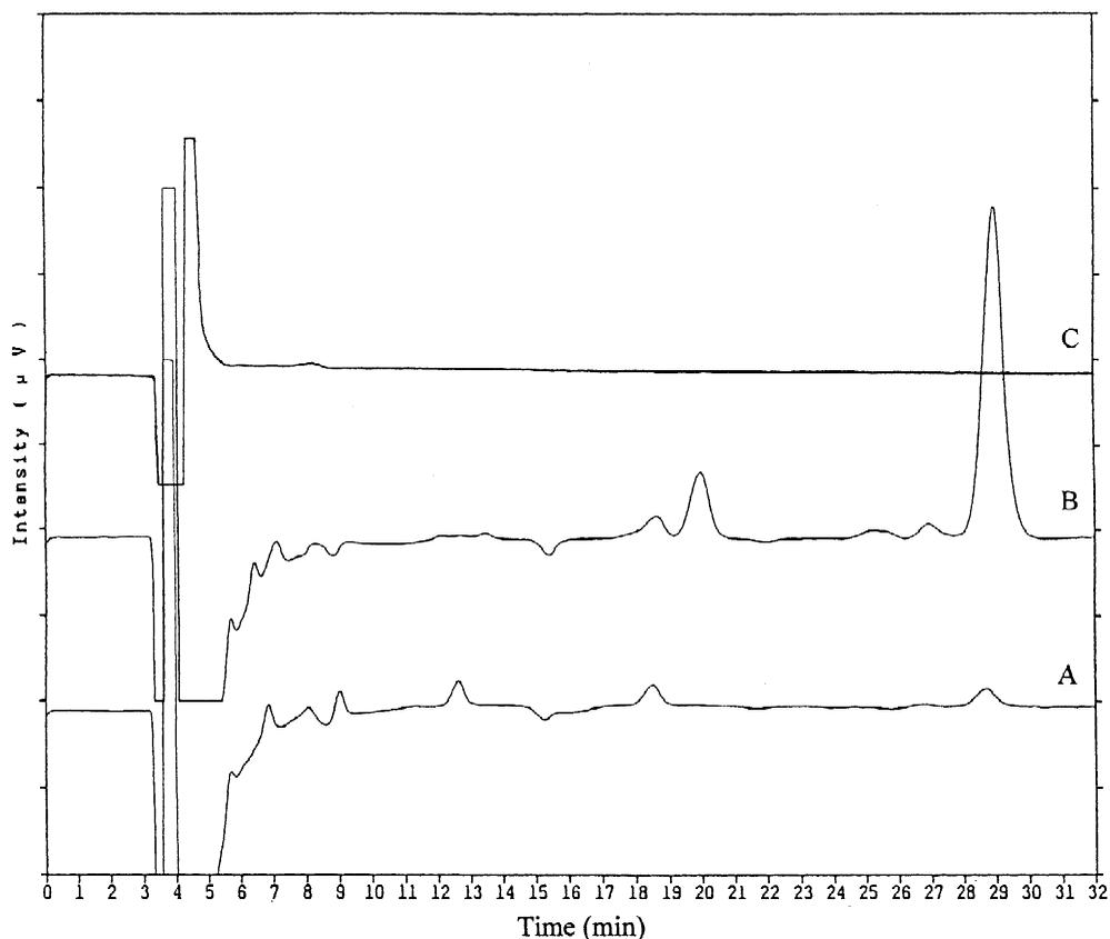
Fig. 5. (A) Chromatogram of a mixture of six iodoalkane standards at 1 ppb (for iodine basis) by using HPLC- $h\nu$ -ED. (B) Chromatogram of HPLC- $h\nu$ -ED assay for real sample 5. (C) Chromatogram of HPLC-ED assay for real sample 5 (lamp off). Chromatographic conditions as in Section 2.4.
