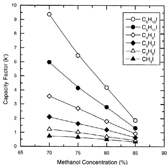
Fig. 2. Effects of methanol concentration on capacity factor ( $k'$ ). Symbols: (▲) iodomethane; (△) iodoethane; (◆) 1-iodopropane; (◇) 1-iodobutane; (●) 1-iodopentane; (○) 1-iodohexane. Other conditions as in Section 2.4.
