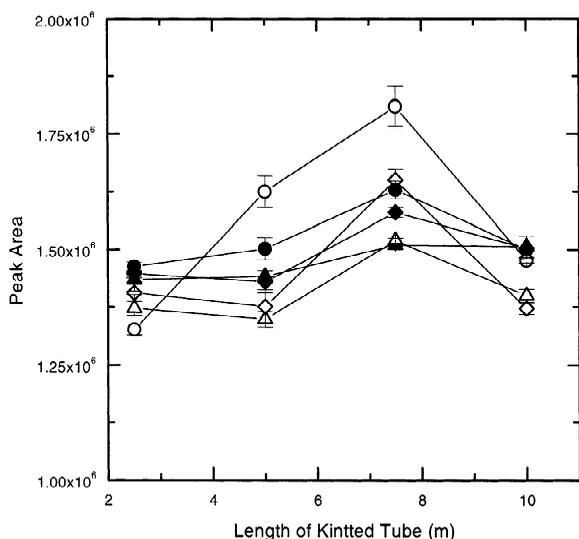
Fig. 3. Effects of reaction coil length on peak area. Notations as in Fig. 2. Each standard is at 10 ppb (for iodine base). Other conditions as in Section 2.4.
