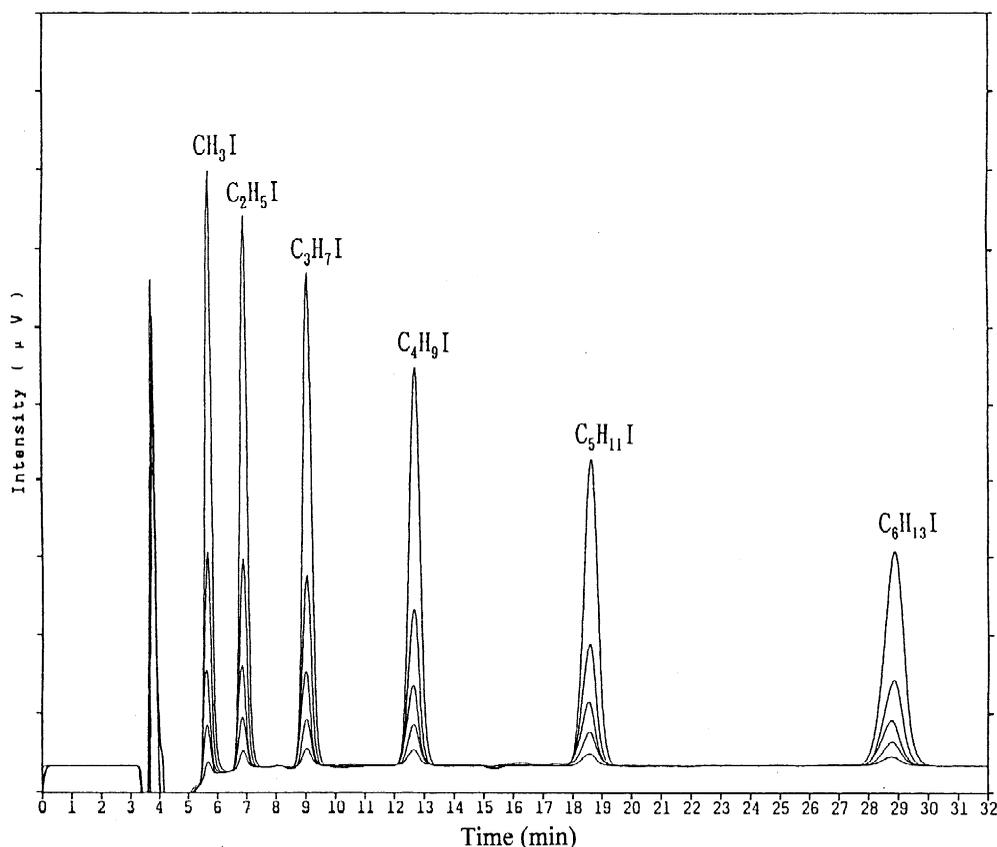
Fig. 1. Chromatograms of a mixture of six iodoalkane standards under five different concentrations 4, 10, 20, 40, and 100 ppb (for iodine basis) by using HPLC– $h\nu$ -ED. Chromatographic conditions as in Section 2.4.
