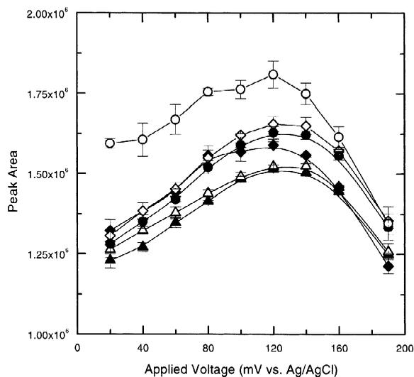
Fig. 4. Effects of applied voltage on the ED response. Notations as in Fig. 2. Each standard is at 10 ppb (for iodine base). Other conditions as in Section 2.4.
